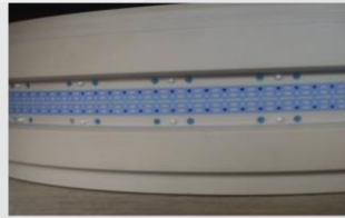
Spot-electroplating The minimum accuracy of gold plating 0.5mm+0.2mm-0mm
